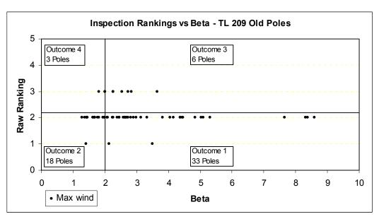
Fig. 1 Summary Plot For Suspension Structures (Pole Bending) –Beta Values Versus Condition Ranking
