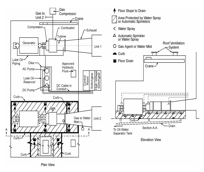
Figure 2.2 Local protection layout for unenclosed combustion turbines and generators
