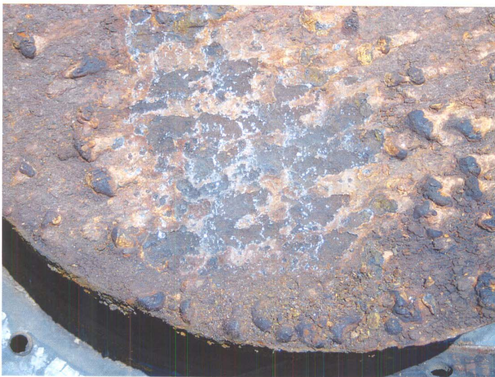
Pitting on Inside Surface of Manhole Cover
