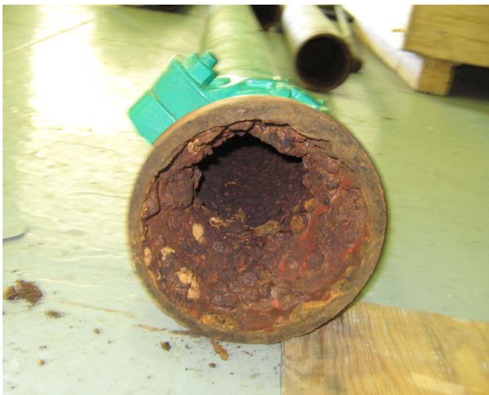
Figure 1. Fouled Cooling Water Pipe, Bay d'Espoir Unit 1 or Unit 2 Spring 2008
