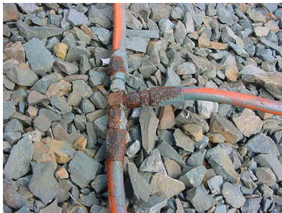
Figure 4: Corroded Synflex Hose Fittings.
