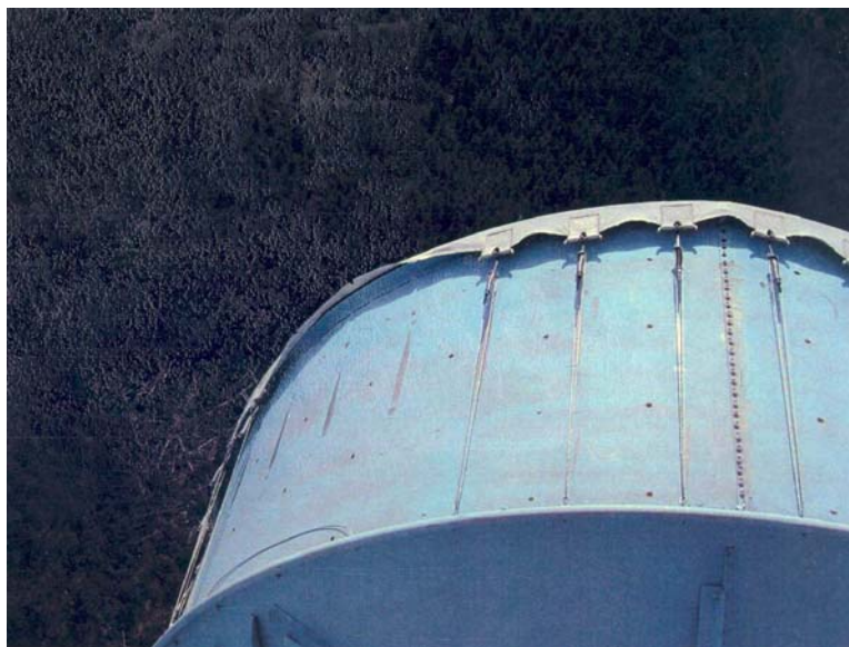
Figure 4: Missing Radome Mounts
