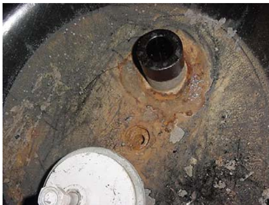
Figure 1: Corroded Air Blast Circuit Breaker
