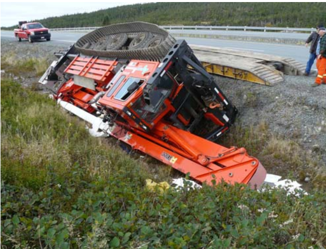
Figure 1: Go-Track unit resting on damaged outriggers and boom.
