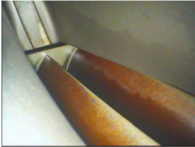
Figure 3: Corrosion on End B Engine
