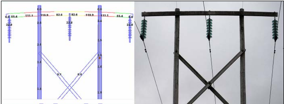
Figure 5: Typical Crossarm Loading under a 31.75 millimetres Ice Load
