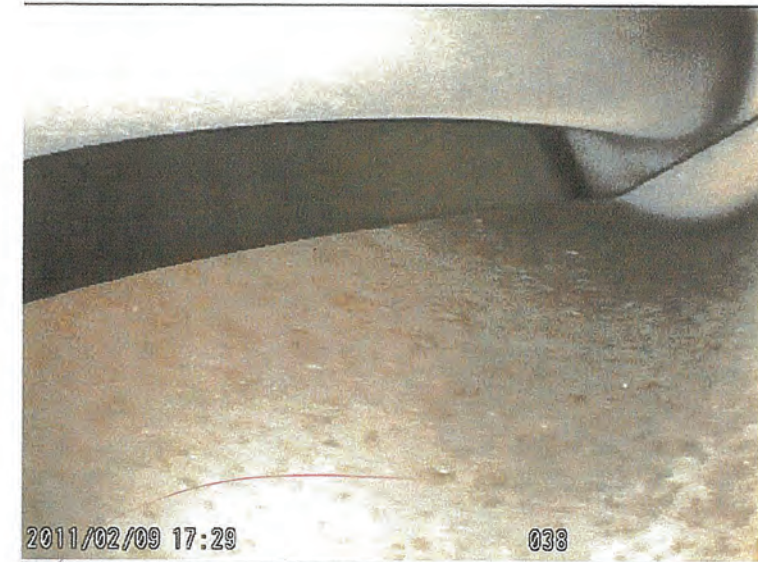
Photo 9. Showing corrosion on blades.
