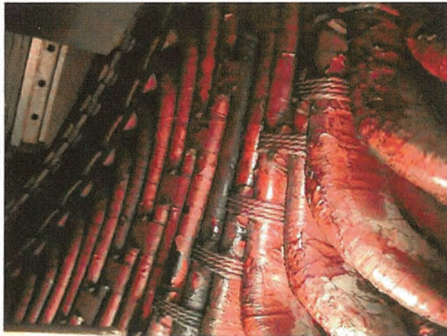
Dry brittle flaking insulation on coils
