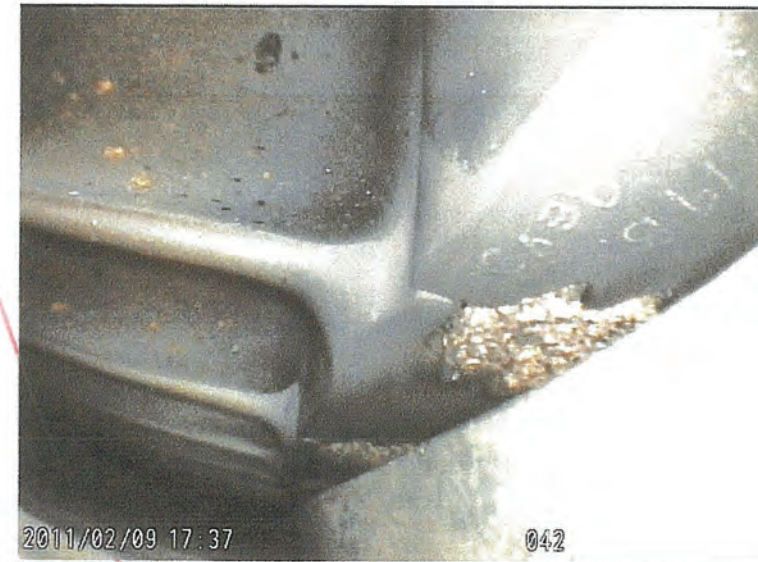
Photo 10. Showing fir tree root corrosion
