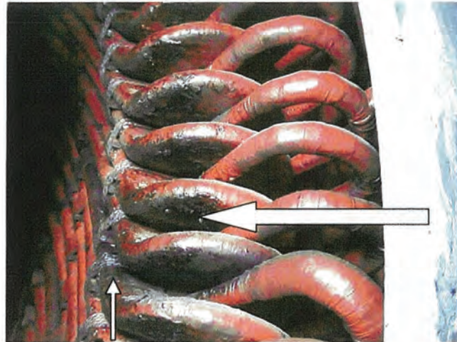
Over heating has occurred in the past: discoloration and resin melted at knuckles.
