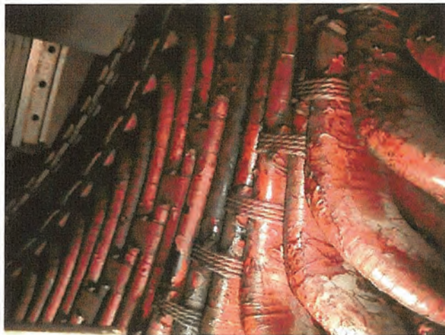
Dry brittle flaking insulation on coils
