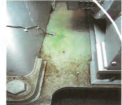
Leakage on bearing foundation
