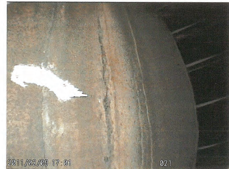
Photo 2. Showing crack around circumference of the PT cone.
