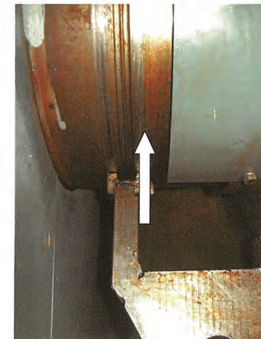
Outboard labyrinth seal and shaft seal (grooves wear marks)
