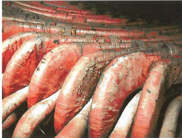
Dry brittle insulation
