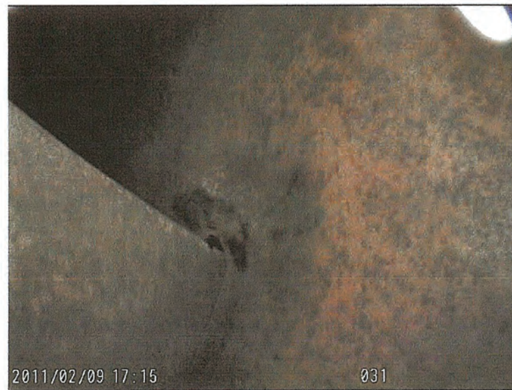
Photo 4. showing weld repair on cone spoke inner edge.
