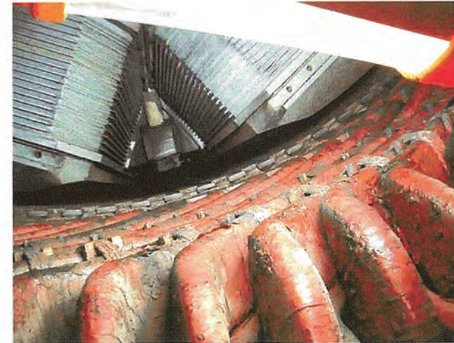
Connections between poles appear in good condition.
