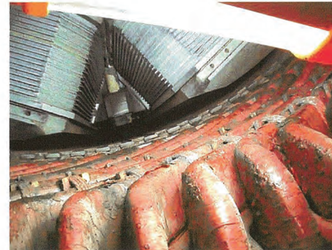
Connections between poles appear in good condition.
