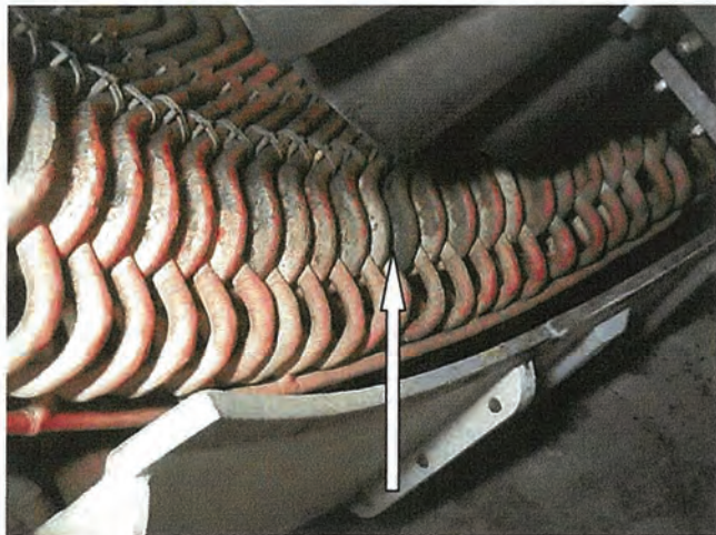
Discoloration heating pattern on some coils.
