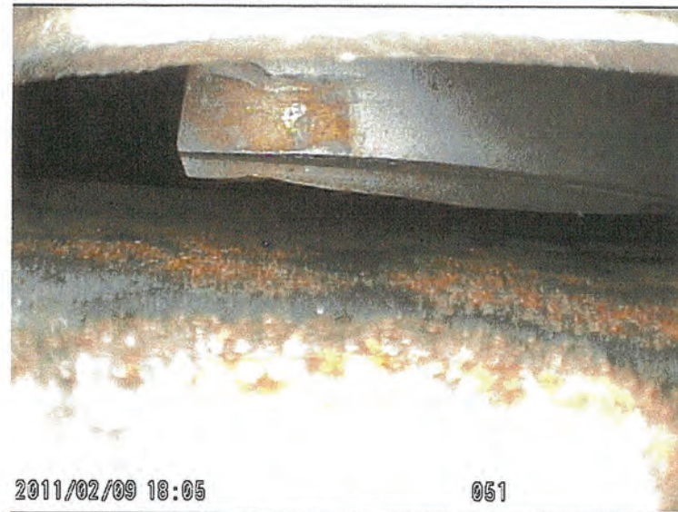
Photo 7. Showing worn blade tips.
