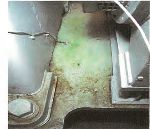
Leakage on bearing foundation
