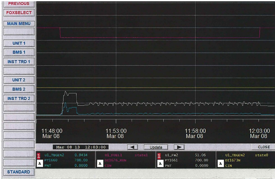
Figure 3: DC lube oil pump test with tank control valve wide open. Magenta is the start/run status of the DC lube oil pump. White is the lube oil pressure in the tank (expect higher value as there is approximately 42 feet of vertical head between the tank and the turbine-generator). Blue is the pressure in the front standard of the turbine-generator. Note the same cyclic pattern in the pressure trend as in Figure 2.
