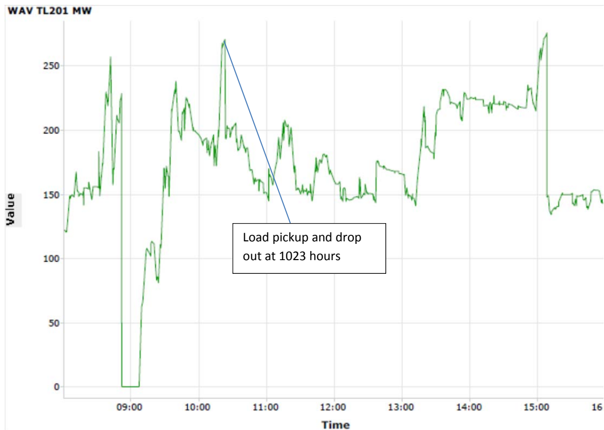
Figure 3-17: TL201 MW Loading from 0800 to 1600 Hours
