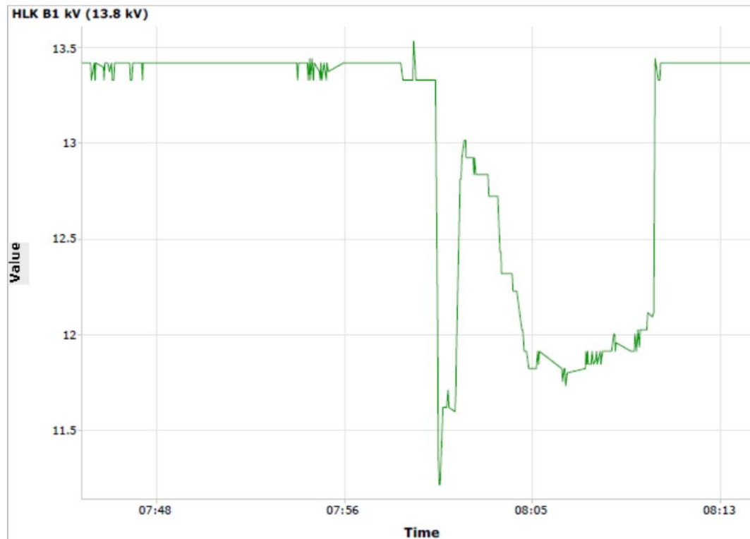
Figure 3-9a: Hinds Lake Terminal Voltage from 0745 to 0815 Hours
