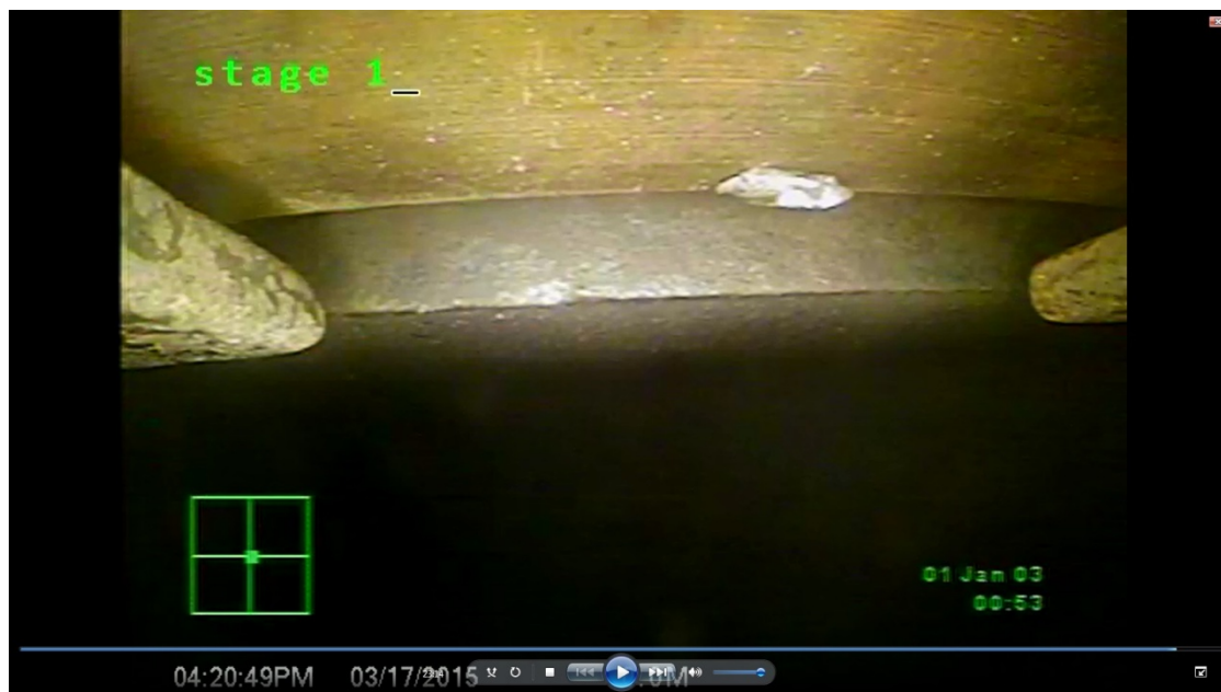
Power turbine with debris visible
