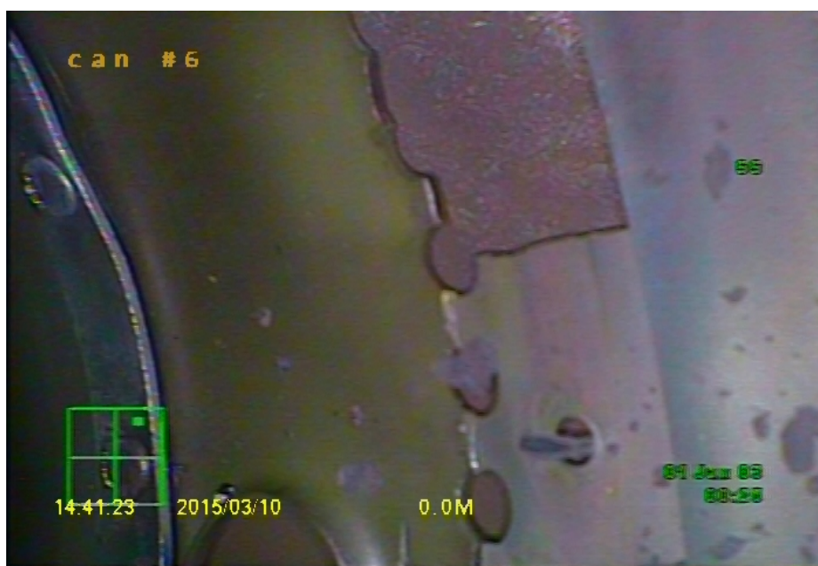
Damage to combustion chamber #6 (large piece missing)
