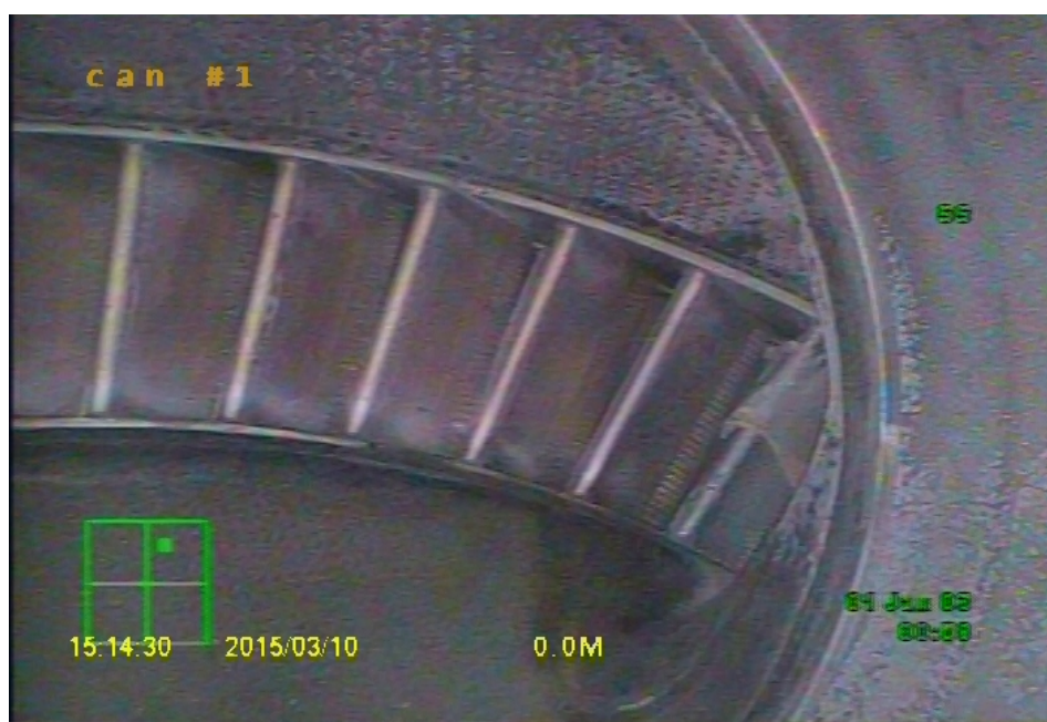
Debris visible in HP turbine as seen through combustion chamber #1
