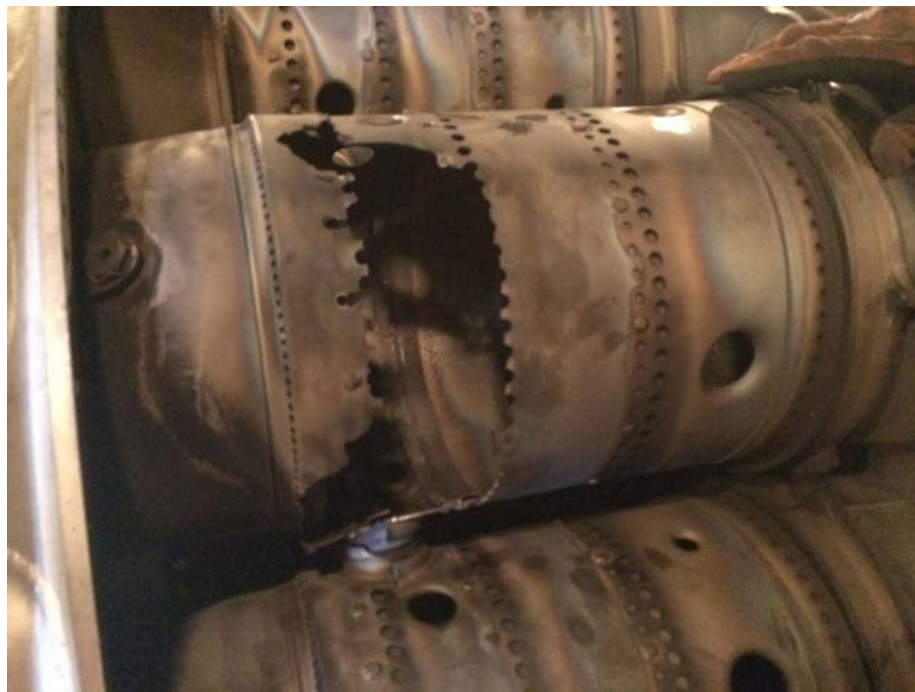
Combustion chamber #8 damage
