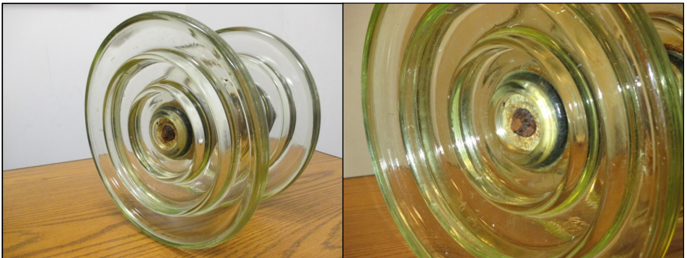
Figure 2: TL203 – Structure 163 Pilkington Insulator Pin Corrosion
