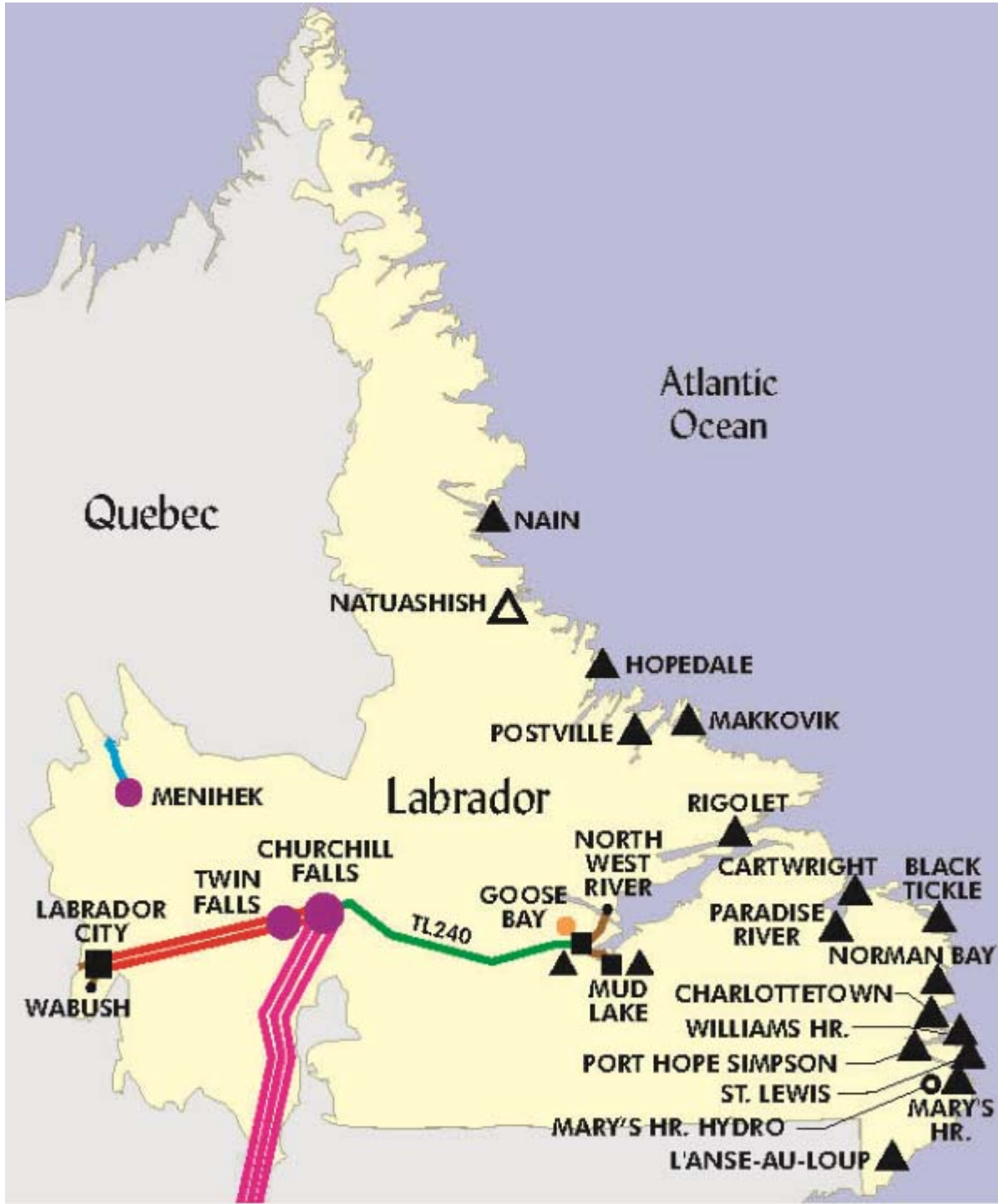
Figure 1: Labrador Generation and Transmission Grid
