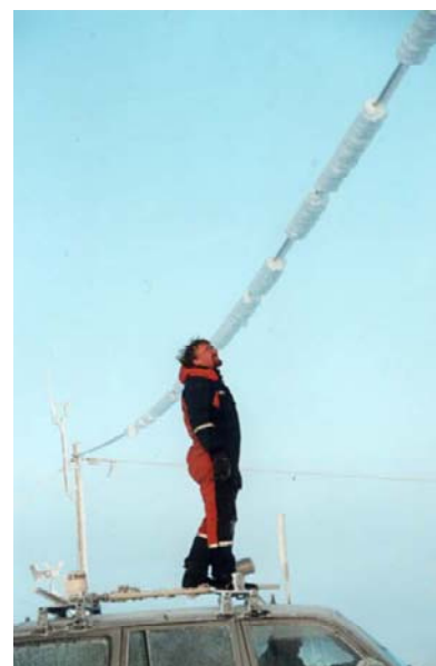
Figure 20. Icing on a vertical rotating circular element. Figure 21. Icing on a horizontal test span.
