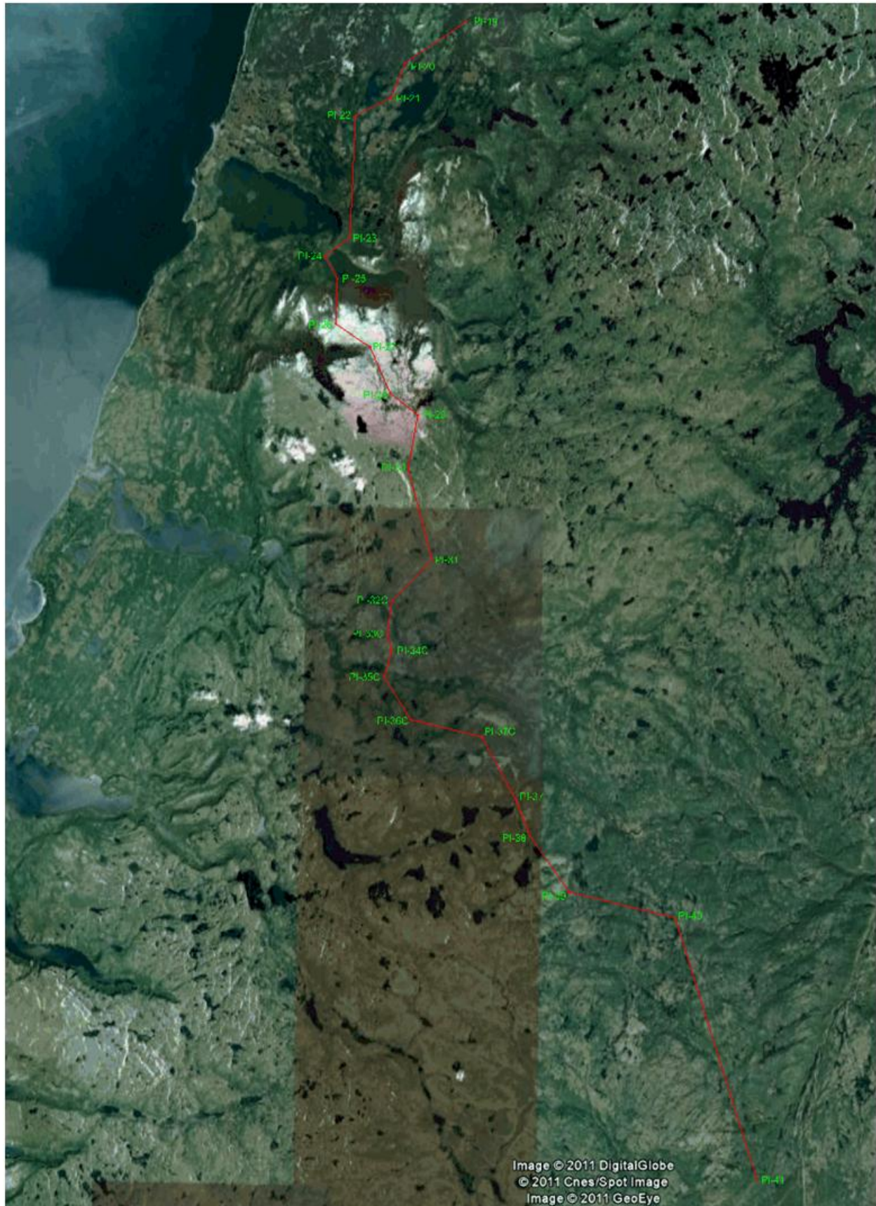
Figure 78. Line route with angle points, PI, marked. Ref. to Table 18.
