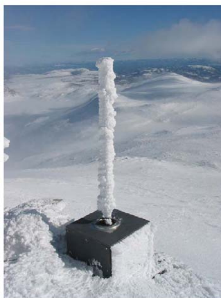
Figure 20. Icing on a vertical rotating circular element. Figure 21. Icing on a horizontal test span.
