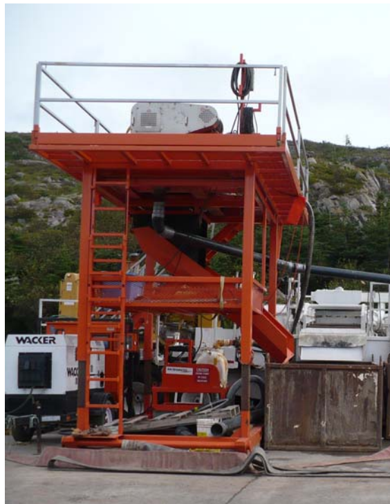
Figure 2-9: Centrifuge Unit - Used for Separating Clay-Size Cuttings
