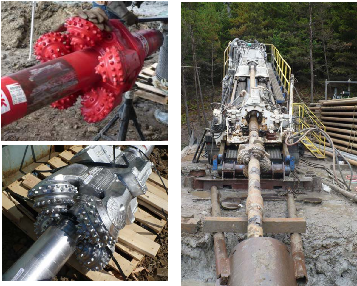
Figure 2-10: Photographs of Typical Hole Openers used to Excavate Bedrock Materials
