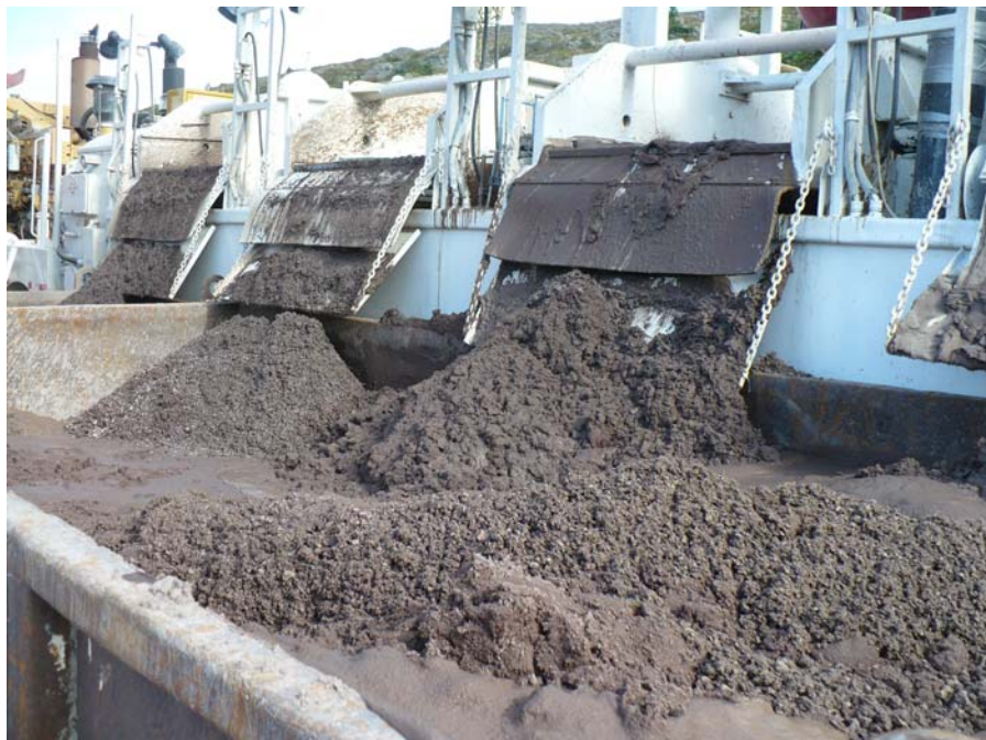
Figure 2-5: Photograph of Typical Spoil Piles after Processing by Separation Plant
