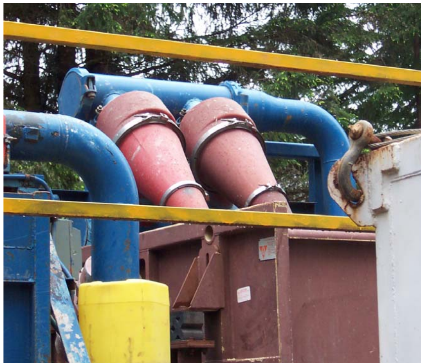
Figure 2-7: Sand Hydrocyclones - Used for Separating Sand-Size Cuttings
