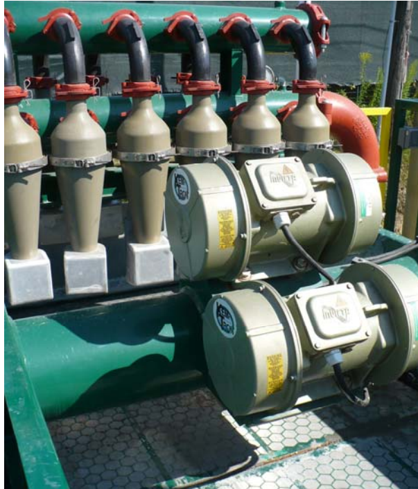
Figure 2-8: Silt Hydrocyclones - Used for Separating Silt-Size Cuttings
