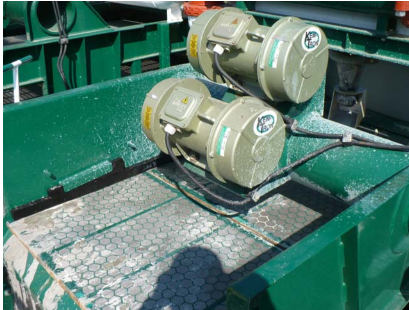
Figure 2-6: Coarse Screen Scalper - Used for Separating Coarse-Size Cuttings
