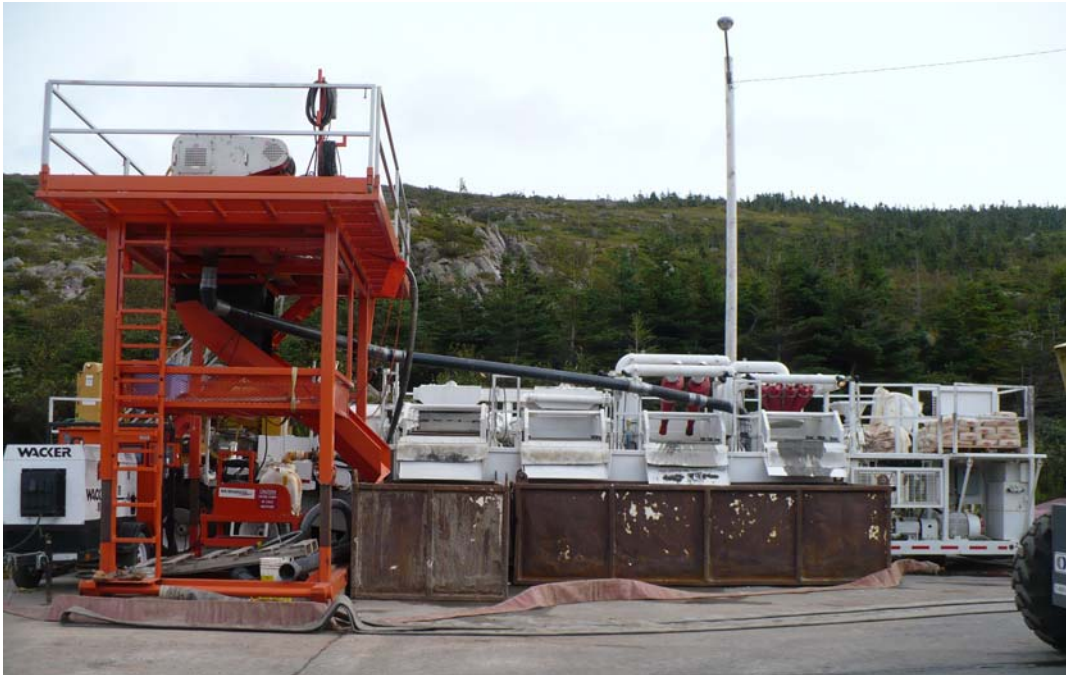
Figure 2-4: Photograph of Typical Separation Plant used to Process Drilling Fluid Returns
