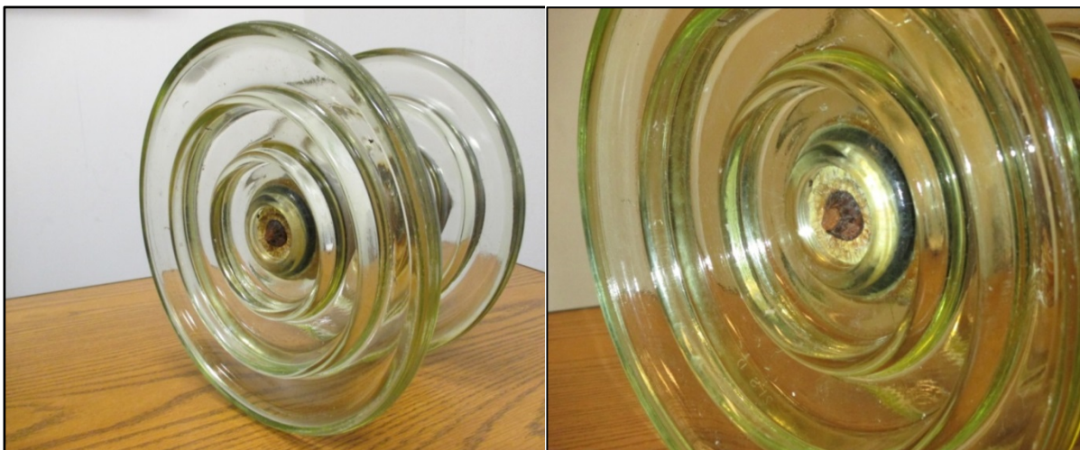
Figure 2: TL-203 – Structure 163 Pilkington Insulator Pin Corrosion
