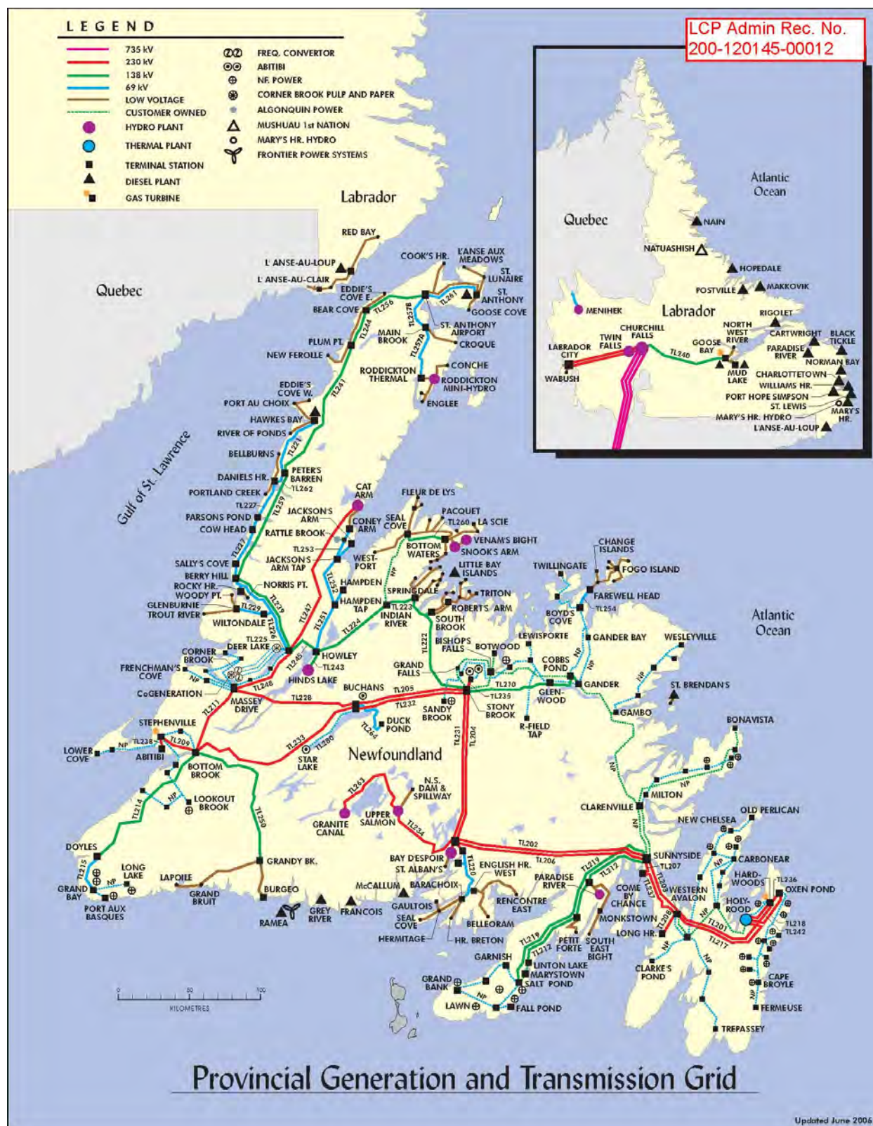
Figure 1-2: Provincial Transmission Grid
