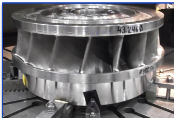
New energy efficient turbine runner for New Chelsea plant.
