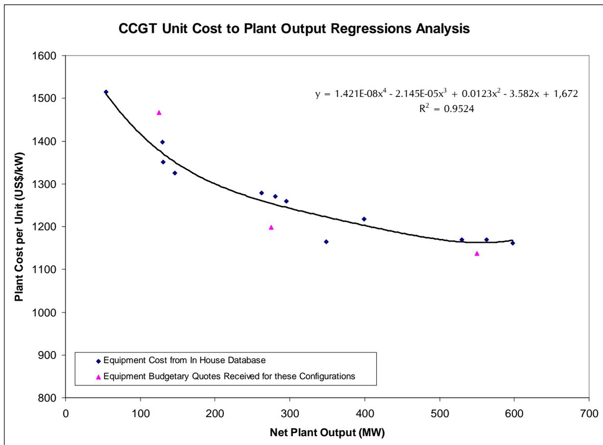
Figure 6.1 - Regression Analysis of CCGT Power Plant Cost Data
