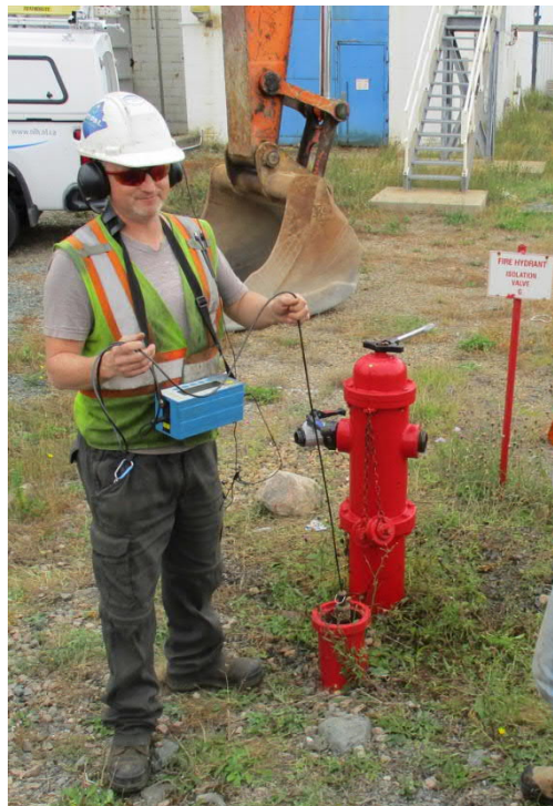
Figure 7-2: Acoustic Testing on Hydrant Gp
