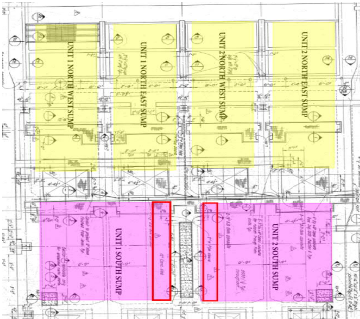
Figure 5-8: Pump House 1 South Sumps: Location of Significant Cracking in Interior Beams
