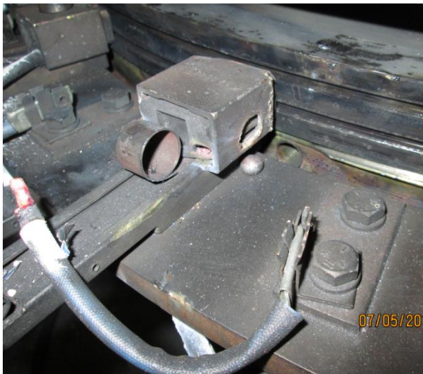
Lead burnt off and brush wear at zero remaining life
