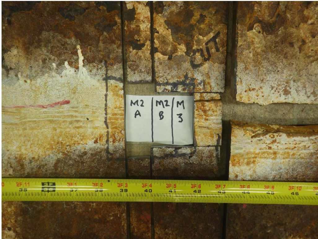
Figure 16 Photograph showing the location of micrographic section the 39 & 42 in. marks
