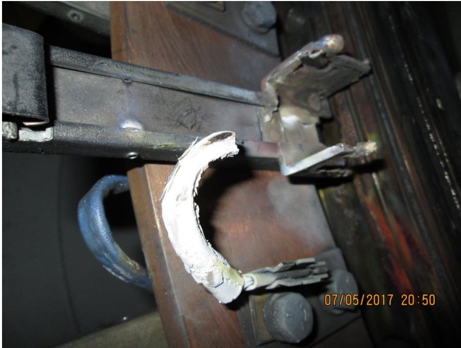
B3: Heavy heat damage to brush, pigtail and holder. The brush wear is less than the threshold for replacement. (Picture 16)
