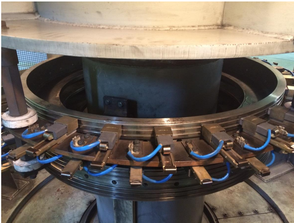
Picture 1: Cleaned slip ring with new brushes and brush holders
