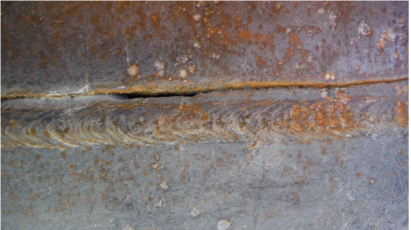
PHOTO 5 – CLOSE-UP OF CRACK. NOTE CORROSION IN CRACK THAT APPEARS OLDER THAN ONE WEEK.
