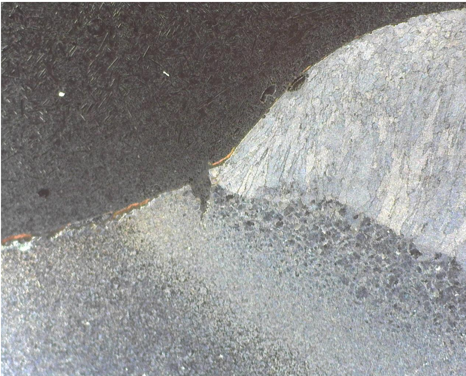
Figure 26 Photograph showing the crack in the MW42 sample at the 42in location after etching
