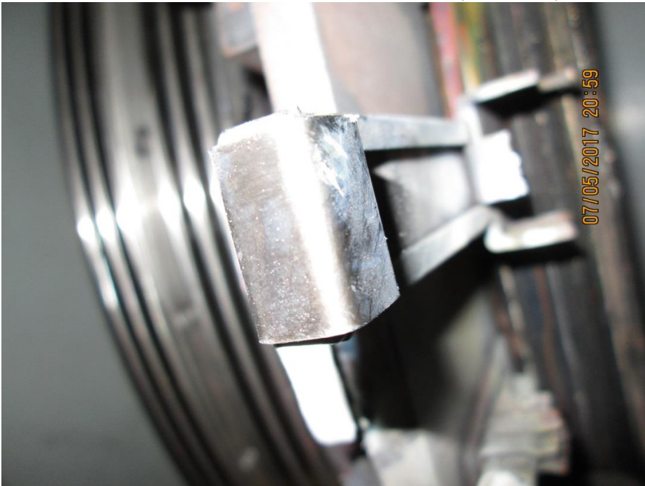
B10: The brush holder melted and the brush fell out. (Picture 23)
