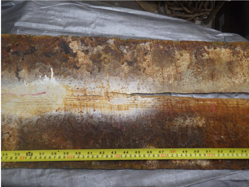
Figure 2 Penstock plate showing one end of the fracture near the 39 inch mark
