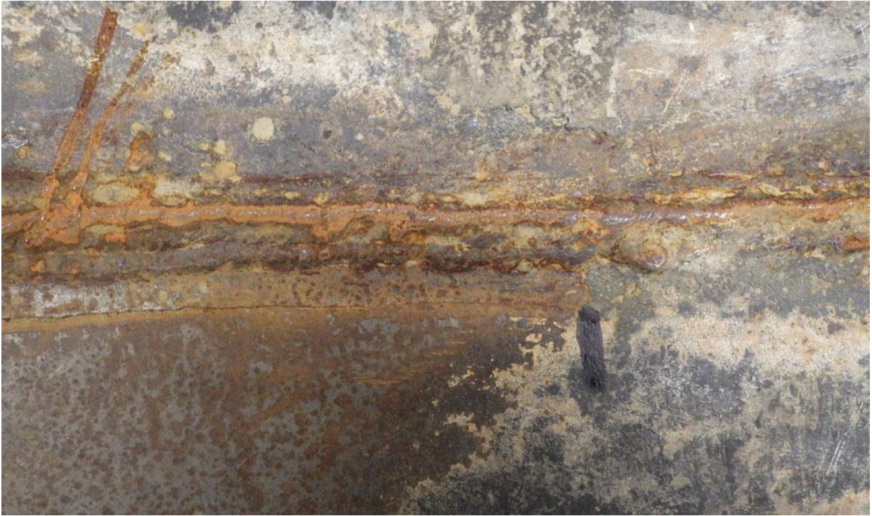
Figure 10 Crack arrest location in base metal offset from weld
