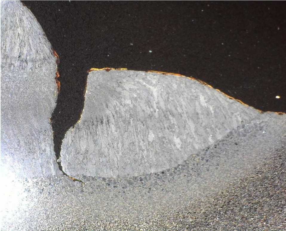
Figure 29 Macrograph showing close-up of the crack in the MW69 sample at the 69in location, etched
