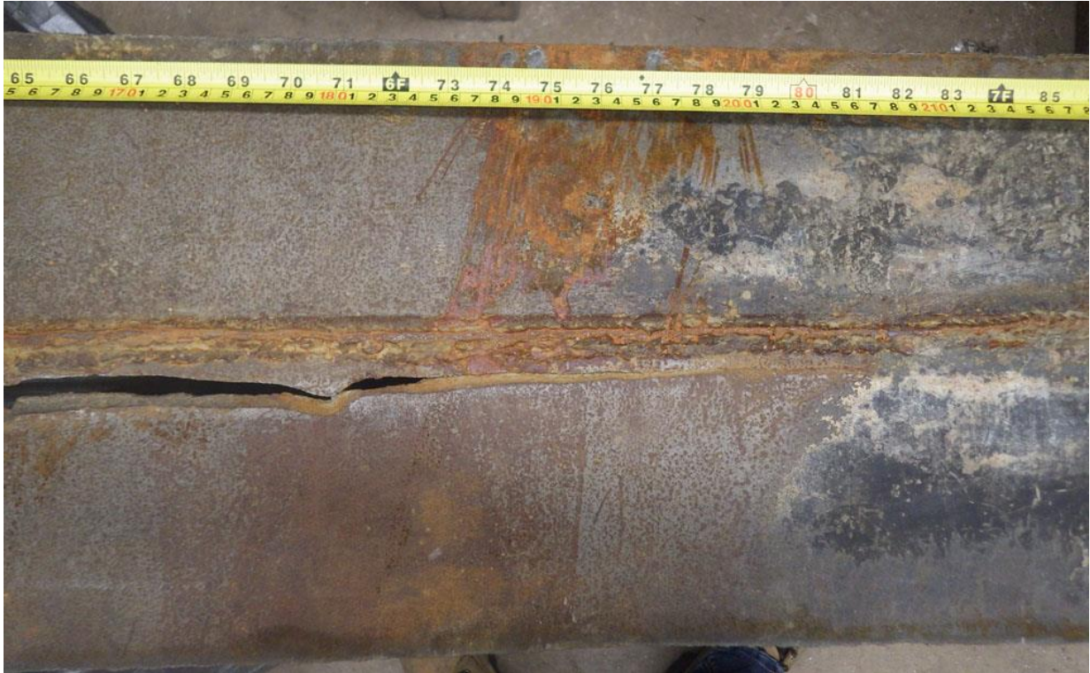
Figure 8 Penstock outside surface showing crack from 65 in. to 82 in.
