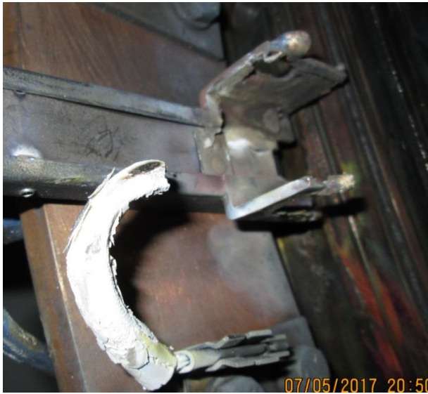
Missing Brush and melted brush holder with lead burnt off
