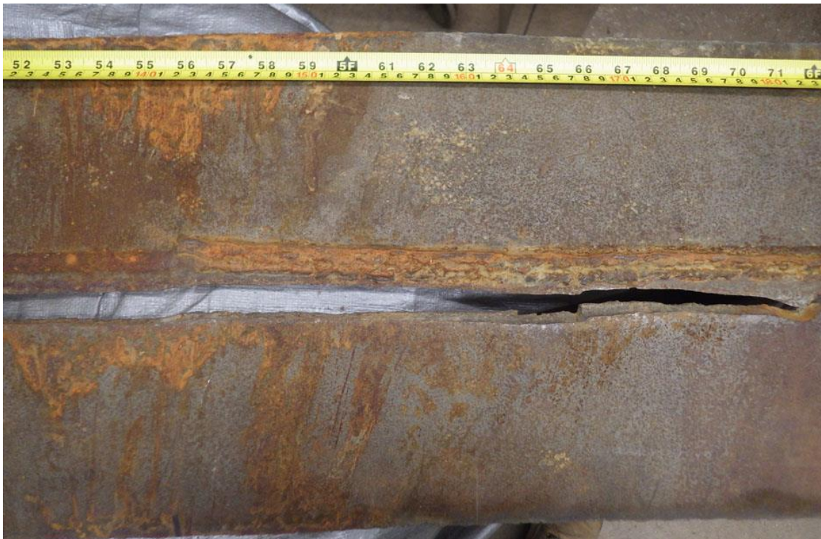
Figure 7 Crack section from the 52 inch mark to the 72 inch mark showing crack travel along the weld.
