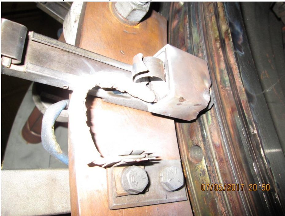
B2: The brush holder melted and the brush fell out. (Picture 15)
