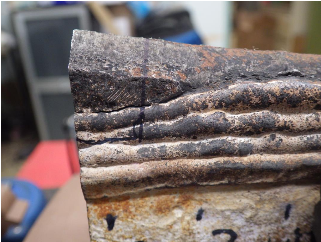
Figure 17 Photograph showing the location of a metallographic sample from near 42in location
