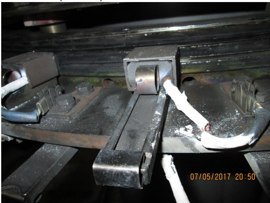
T10: The brush holder has a small melt area on one top corner. The brush wear is at the threshold for replacement. The pigtail insulation is melted through and copper is intact. (Picture 13)
