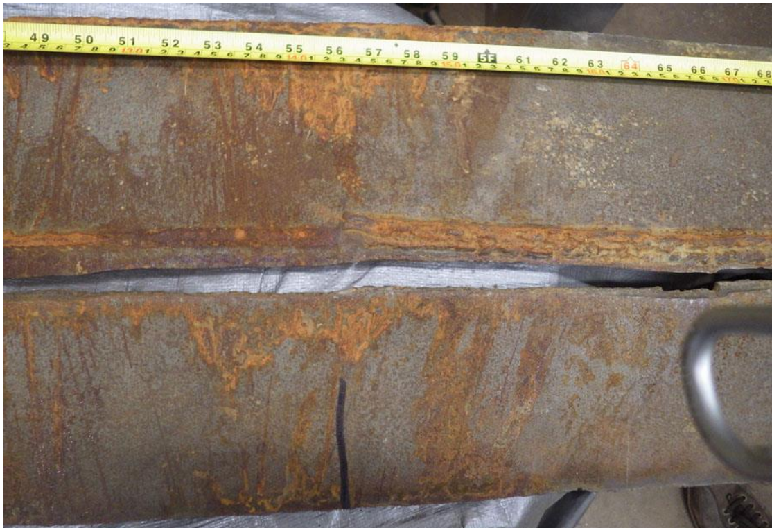
Figure 9 Crack near the transition of original weld and repair weld
