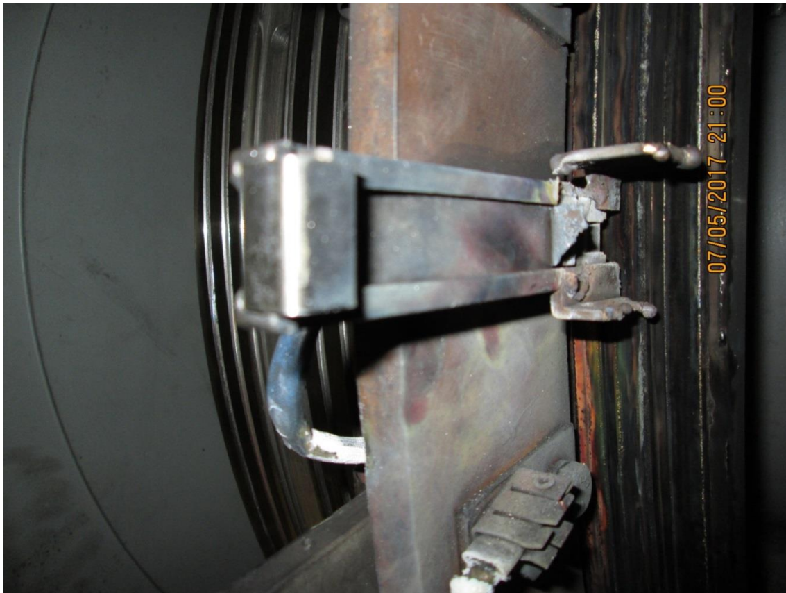
The insulator near the cable connection to the slip ring has splatter damage. (Picture 24)
