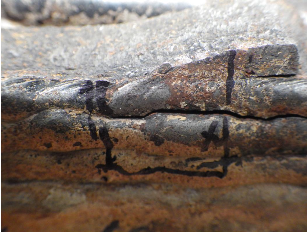
Figure 18 Photograph showing the location of a metallographic sample from near 69in location
