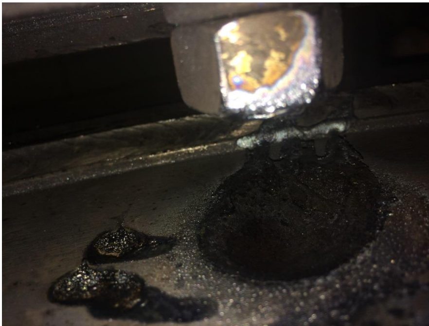
Close-up of a flashover point between the slip rings
