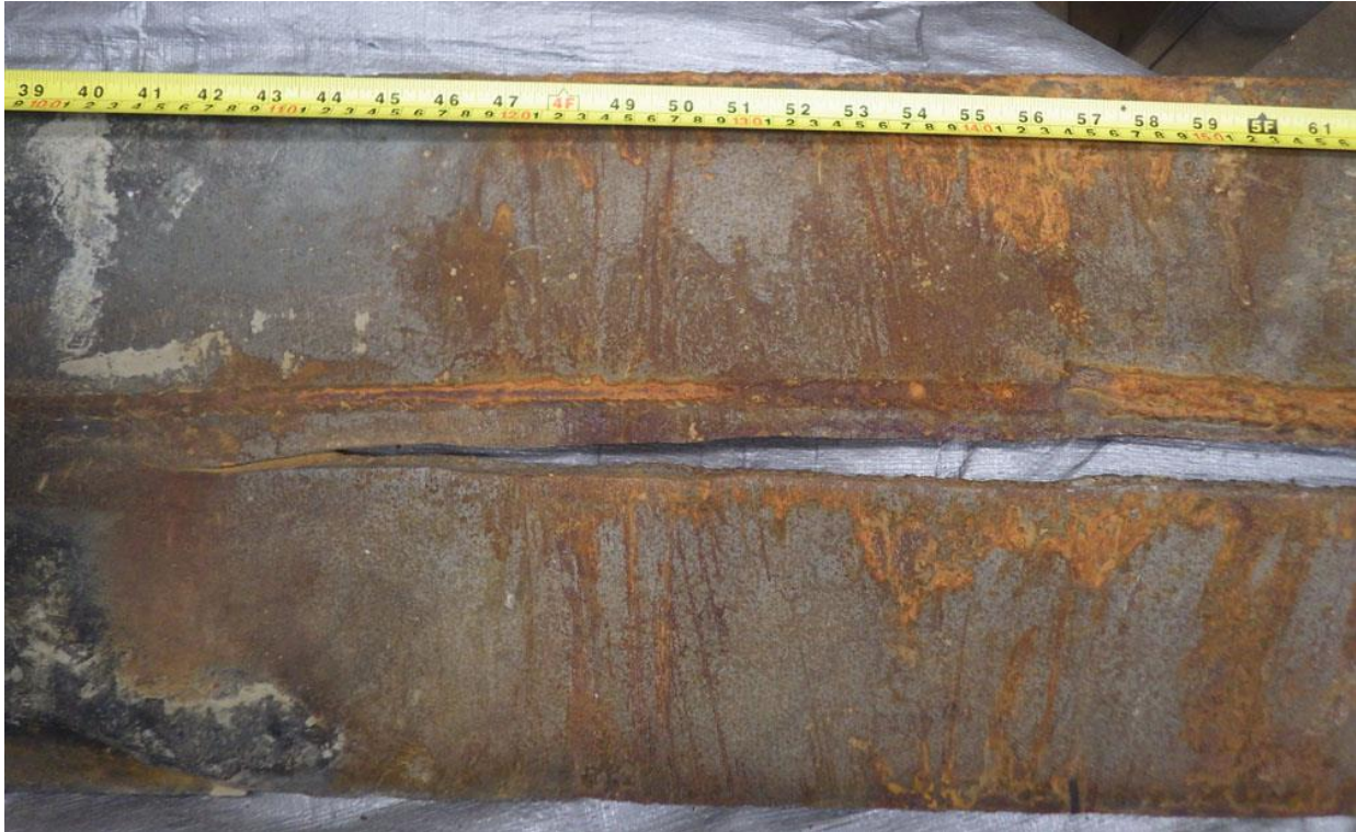
Figure 6 End of the crack on the outside of the Penstock showing the crack arrest in the base metal.
