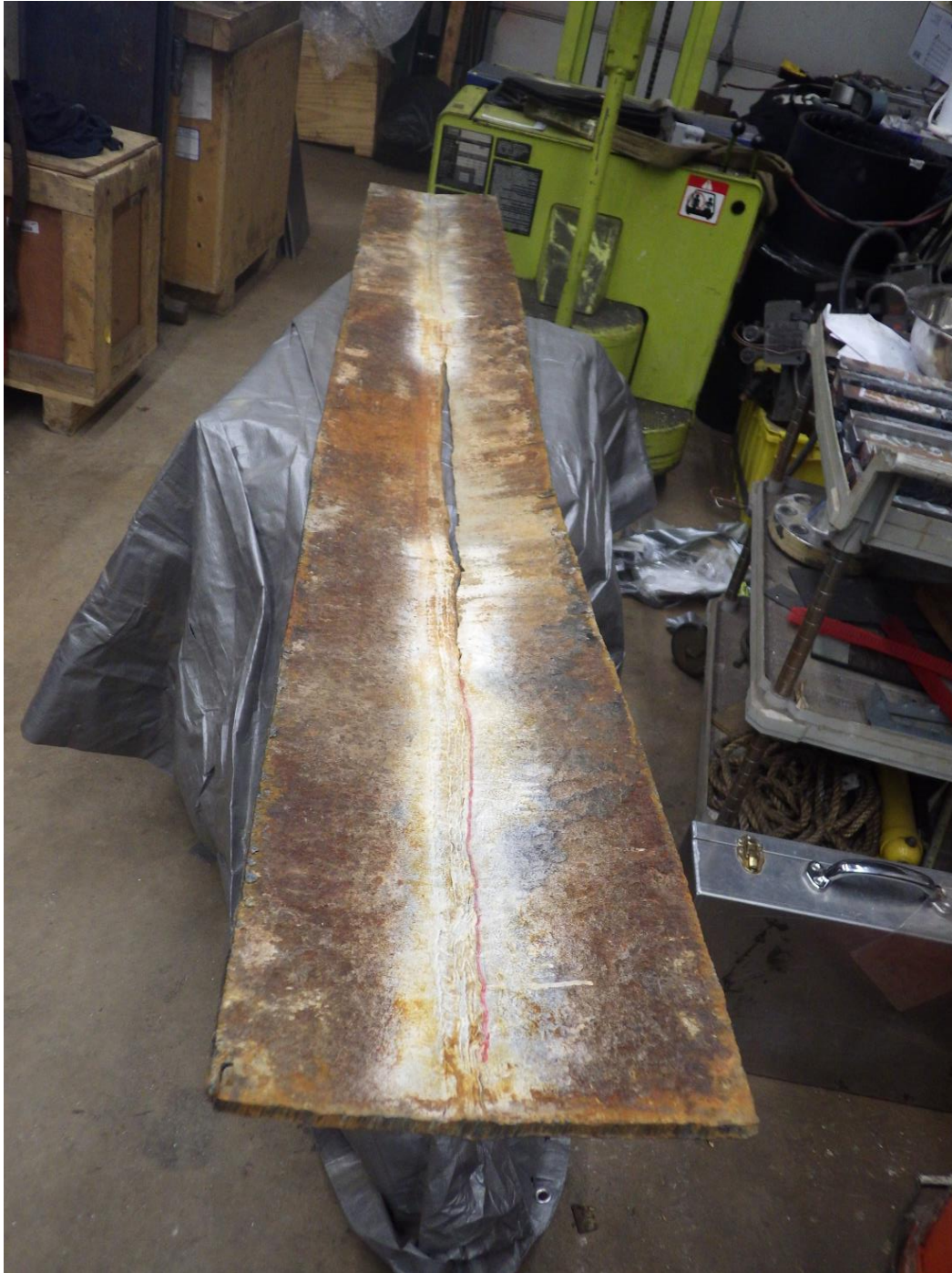
Figure 1 Failed Penstock plate as received
