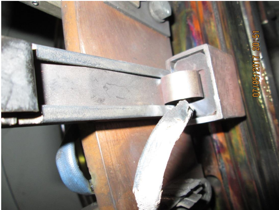
B3: Heavy heat damage to brush, pigtail and holder. The brush wear is less than the threshold for replacement. (Picture 16)
