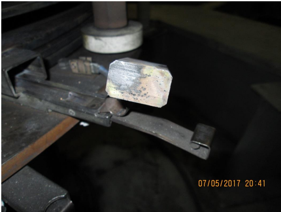
T2: The brush holder has some metal loss on the surface adjacent to the ring. The brush wear is a little below the threshold for replacement. The pigtail is melted off at the brush connection. (Picture 4)
