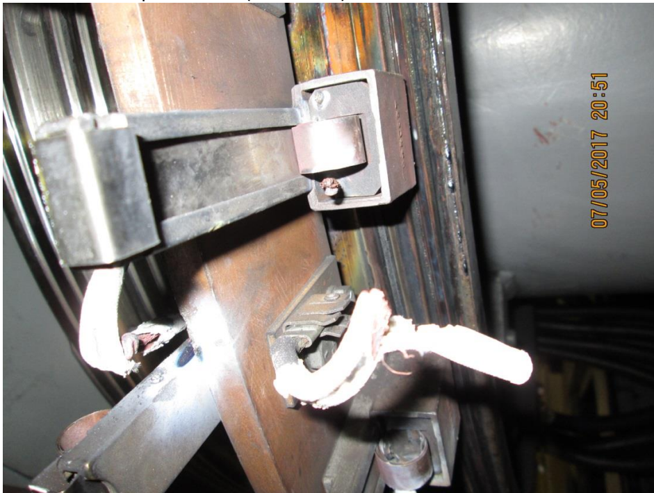
B5: Heavy heat damage to brush, pigtail and holder. The brush wear is less than the threshold for replacement. (Picture 18)
