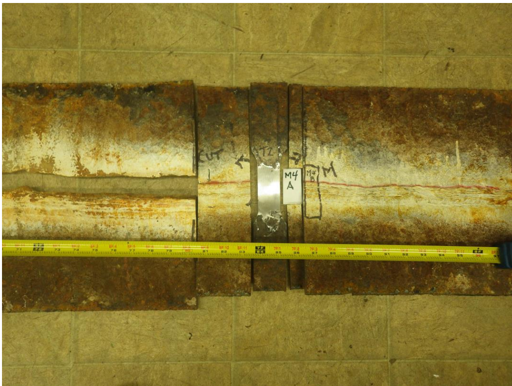
Figure 15 Photograph showing the location of Tensile 2, Macros M4A & M4B between the 72 & 75 in. marks
