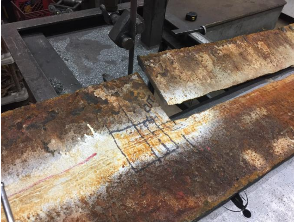
Figure 12 Photograph of the plate as it was being sectioned showing deformation due to residual stresses
