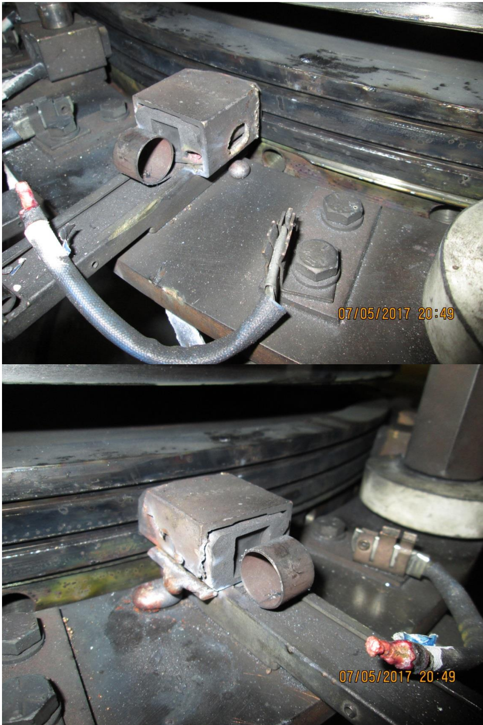
T8: The brush holder has pits / splatter on the top, and some metal loss on the surface adjacent to the ring. The brush wear is at the threshold for replacement. The pigtail is melted off in the middle (between the brush and the connector). The spring is broken. (Picture 11)
