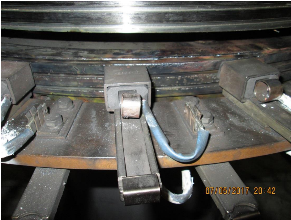
T4: There is minor damage to the brush holder. The brush wear is at the threshold for replacement. The pigtail is melted off in the middle (between the brush and the connector). (Picture 6)
