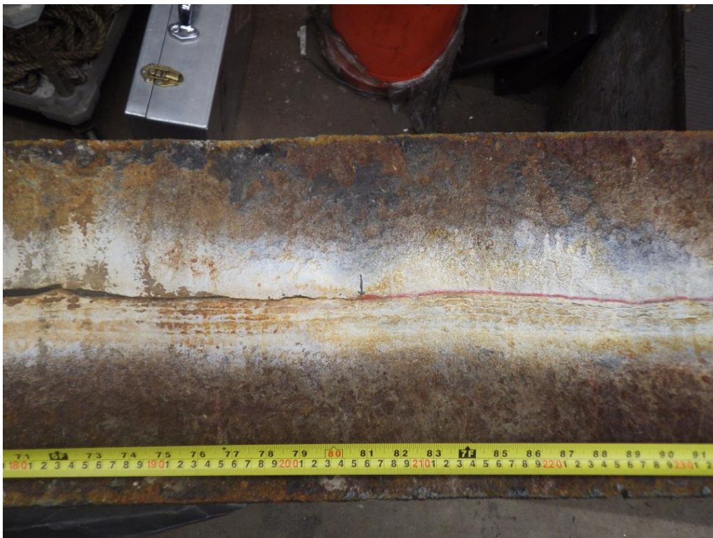
Figure 5 Crack in the plate from the 70 inch mark to the end of the crack near the 82 inch mark
