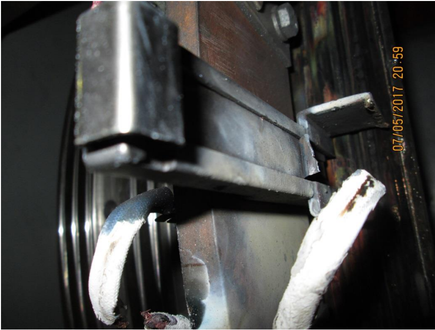
B9: The brush holder melted and the brush fell out. (Picture 22)
