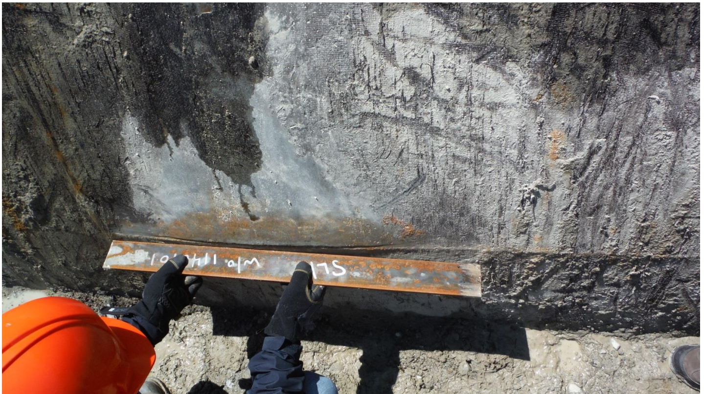
PHOTO 4 – USING STRAIGHT BAR TO HIGHLIGHT BULGE IN PENSTOCK PLATE
