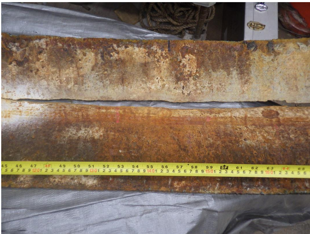
Figure 3 Crack in the plate from the 45 inch mark to the 65 inch mark
