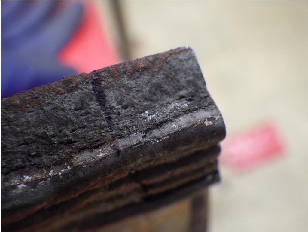
Figure 20 Photograph showing the location of a metallographic sample from near the 79 in. marks
