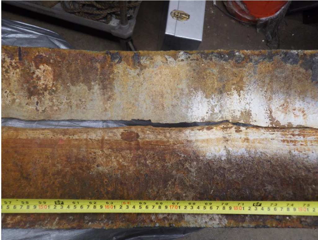
Figure 4 Crack in the plate from the 57 inch mark to the 75 inch mark
