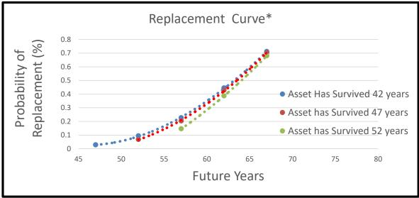
Figure 4: Replacement Probability of the X-Arm Plant Assets<sup>5</sup>
