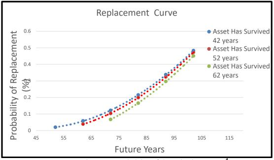
Figure 3: Replacement Probability of the Pole Plant Assets<sup>4</sup>
