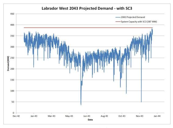
Figure 3 – Labrador West Projected Load Profile for 2043 – System with SC3
