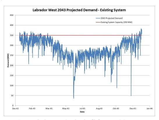
Figure 2 - Labrador West Projected Load Profile for 2043 - Existing System
