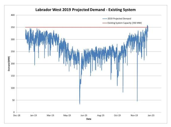
Figure 1 - Labrador West Projected Load Profile for 2019 - Existing System
