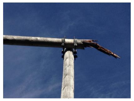
Figure 5: 2017 Outage Crossarm Failed and Broke Free
