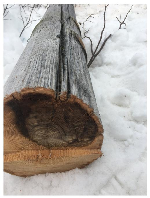
Figure 1: Deep Crack Causing Decay to Centre of Crossarm
