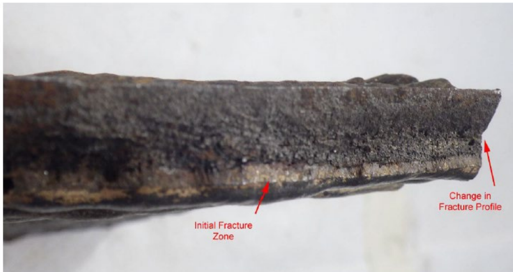
Figure 3-7: Crack propagation modes for 2017 Penstock 1 Failure (Ref. 3)
