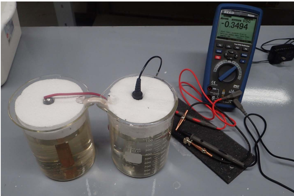
Figure 1 Galvanic Series Test Setup
